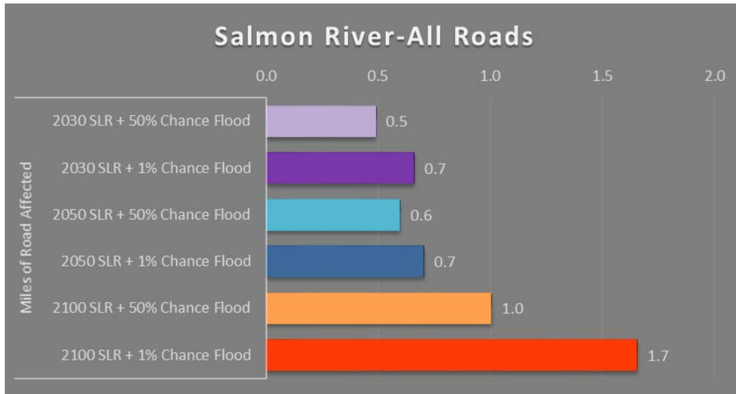
Figure 58. Miles of Road Impacted in the Salmon River Future Flooding Scenarios
